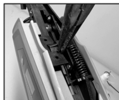
9. Install the left cover plate
