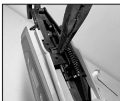
4. Remove the left cover plate
