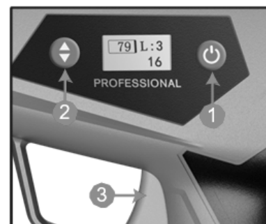
12. Turn on power, press and hold shift button for 1 second then engage trigger
