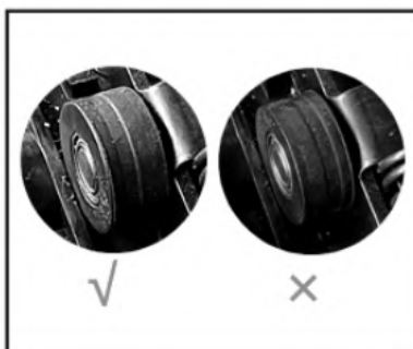
8. Diagram of difference of rubber belts.
