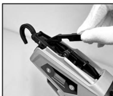
11. Install the pressure strip
