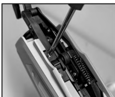
10. Tighten the screws on the left cover plate.
