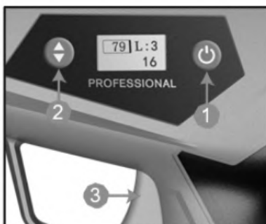
5. Turn on the tyer, press and hold the gear shift button for 1 sec. and then activate the trigger when you hear a sound.
