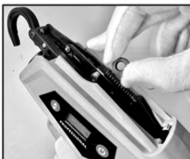
7. Replace the rubber belt with a new one. Make sure the slot in it is facing out.
