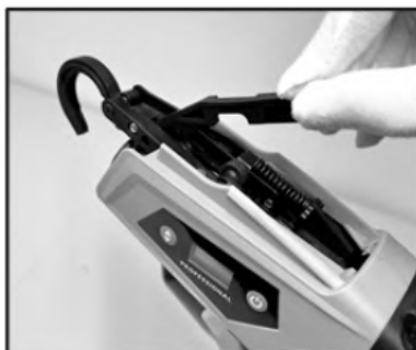
2. Remove the clamp plate.
