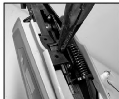
9. Install the left cover plate
