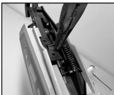
4. Remove the left cover plate
