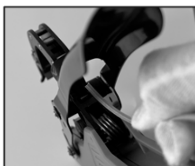
4. Insert the wire from the bottom of the tyer.
